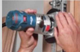
Route Hinge Mortises
